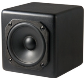
The smaller of the two models, the CR-1, houses a 68mm speaker that screws directly onto the 12mm MDF cabinet. The reasons for this are sonic: edge diffraction was apparently harming the clarity of a test model that was built with a recessed driver.
